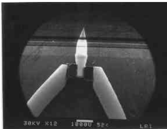
Figure 3.1 A scanning electron microscope (SEM) micrograph of a single carbide cathode in a Vogel-type mount.
