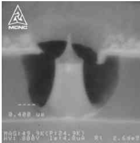
Figure 3.8 A MCNC Si field emission array single tip configuration (courtesy of MCNC).
