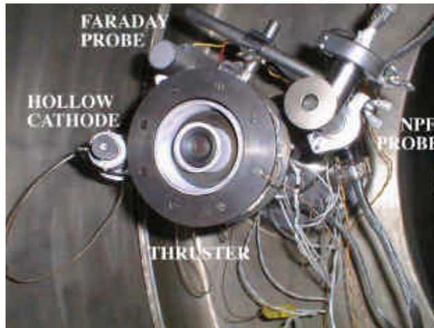
Figure 2.2 The PEPL-70 Hall thruster with a hollow cathode, neutral particle flux (NPF) probe, and Faraday Probe.
