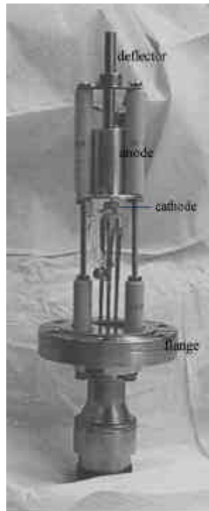
Figure 3.11 The field emission cathode test flange in UHV facility.
