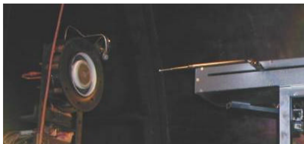
Fig. 4 Typical configuration of the HARP table and the P5 thruster. The picture shows the B-Dot probe in its zero position, which is 150 mm downstream of the thruster exit plane. A sweep of the probe occurs over 180 mm.
