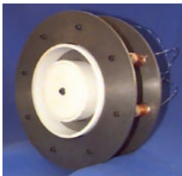
Fig. 2 P5, 5 kW class laboratory model Hall thruster.
