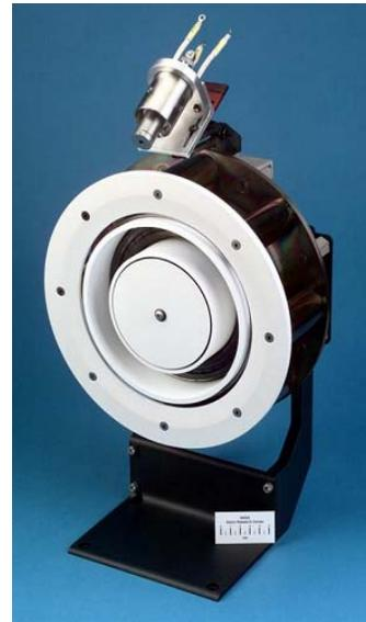
Figure 1. NASA-173Mv1 Hall Thruster
