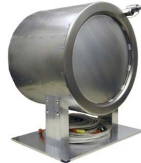
**Figure 2. Laboratory model 4 (LM4) 40-cm NEXT ion thruster.**
