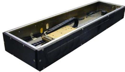
**Figure 4. High-speed Axial Reciprocating Probe (HARP) positioning system.**
