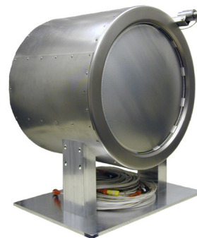
Figure 2. Laboratory model 4 (LM4) 40-cm NEXT ion thruster.
