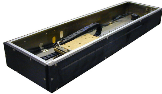
Figure 4. High-speed Axial Reciprocating Probe (HARP) positioning system.
