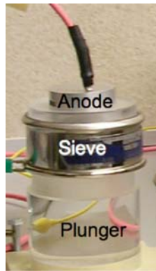
Figure 17: First generation prototype using sieving delivery method.
