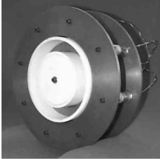
Figure 1: University of Michigan/USAF P5 5 kW Hall Thruster
