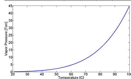
Figure 2: Vapor pressure curve for diatomic iodine.
