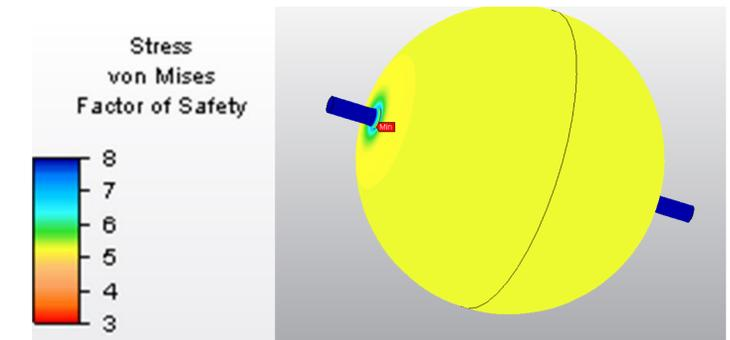
Figure 6: Stress analysis of the spherical titanium tank. The tank can store propellant at 100 atm. Safety factor is shown, but is increased with a rounded fillet at the tube stub juncture.
