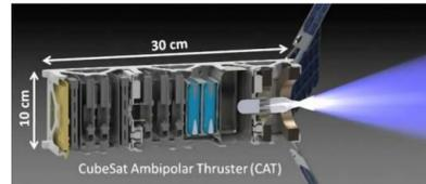
Figure 1: CAD concept drawing of CAT.
