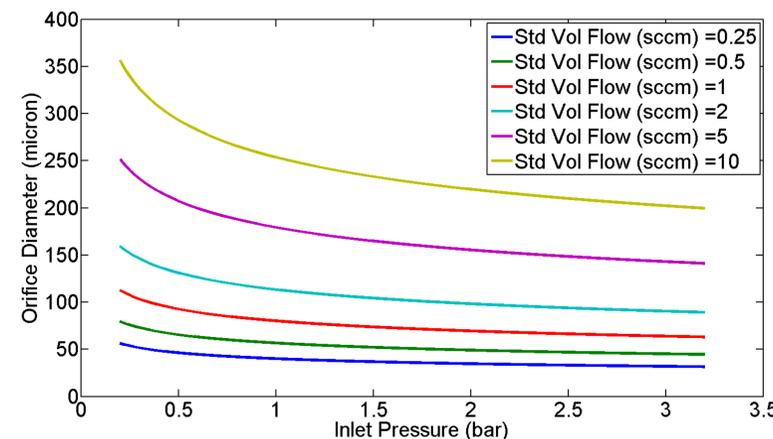
Figure 5: Possible flow conditions using standard static orifice sizes and adjusting the Beswick regulator setpoint.
