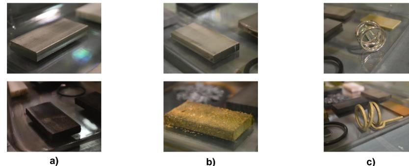
Figure 3: The top image is a control specimen; the bottom is a specimen that has been dosed at STP for 48 hours. a) 316 stainless steel, b) 7075 aluminum, c) silver RF antenna
