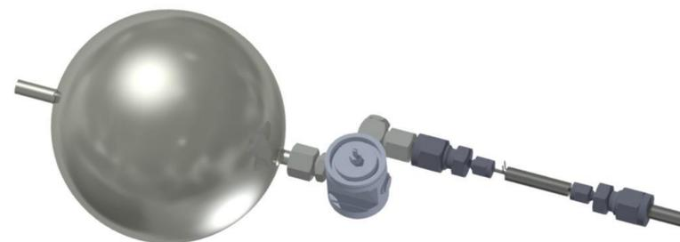
Figure 4: A CAD assembly of the gas-storable propellant feed system.
