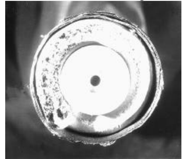
Erosion at outer edges
