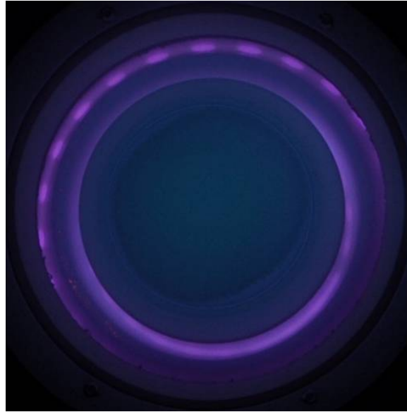
Figure 8. A photograph of a Hall thruster operating at an off-nominal condition, where the discharge is characterized by increased luminescence at uniform intervals around the circumference.
