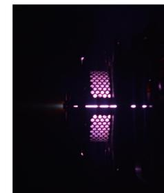
**Figure 4.** CAT firing in the low flow rate, high power mode.
