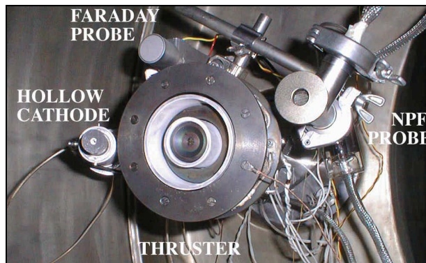
Figure 5 - The 1.4 kW PEPL-70 Hall thruster.
