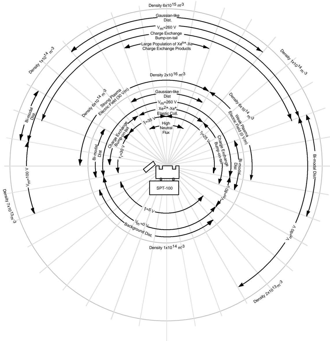
**Figure 8-1. Heavy-particle structure of SPT-100 plume. The SPT-100 body outline including the cathode and support structure is drawn to scale with the 0.5 m and 1.0 m radius arcs shown. Azimuthal increments of 10 degrees are indicated. Quantities lying near the inner circle denote those values at 0.5 m radius, while quantities about the outer circle represent 1.0 m radius values.**
