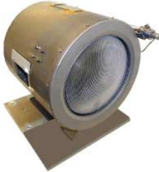
Figure 6.3: Photograph of the FMT-2 ion thruster.
