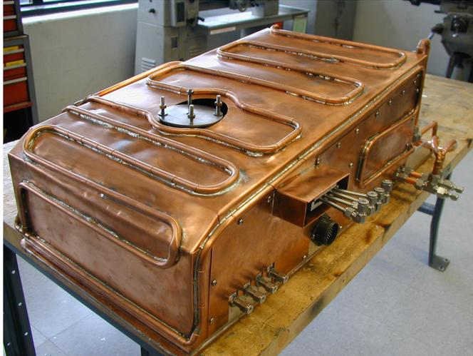
**Figure 2-30: Picture of the NASA-457 Null-type Inverted Pendulum Thrust Stand.**
