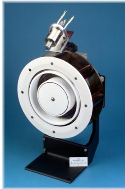
**Figure 2-3: NASA-173Mv1 Hall thruster.**
