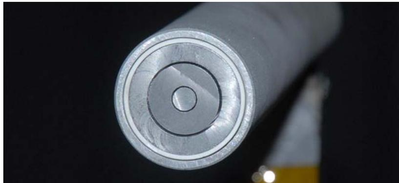
**Figure 3-25** Photograph of the AFRL nested Faraday probe shown in the 0.5 mm gap width configuration.
