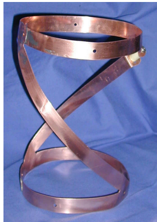
Figure 3.5: Photograph of the double-helix, half-wavelength antenna.
