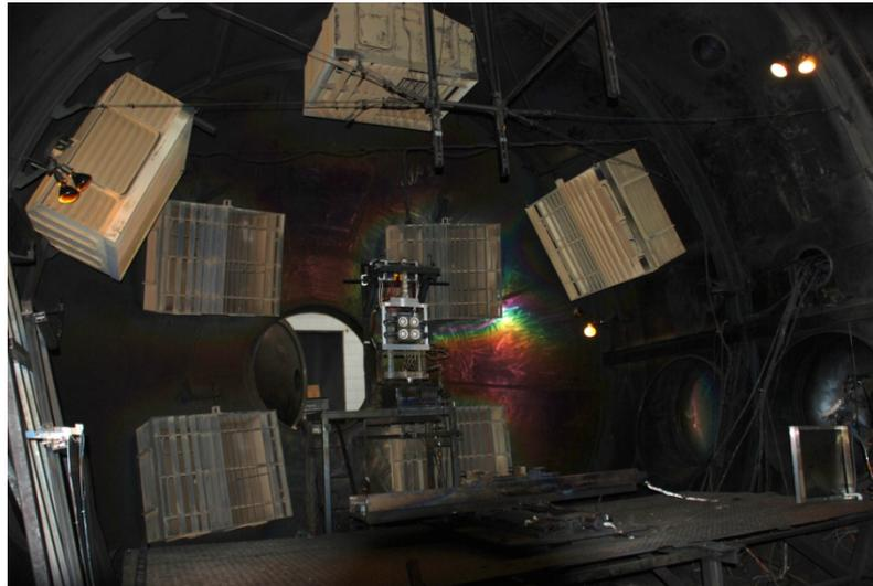
Figure A.2. Internal view of Hall thruster cluster from within the LVTF. Cluster is mounted upon the NASA-type inverted pendulum thrust stand, near the radial center of the vacuum chamber. The seven cryogenic pumps are clearly visible. This photo was taken shortly before pumping down to vacuum conditions.
