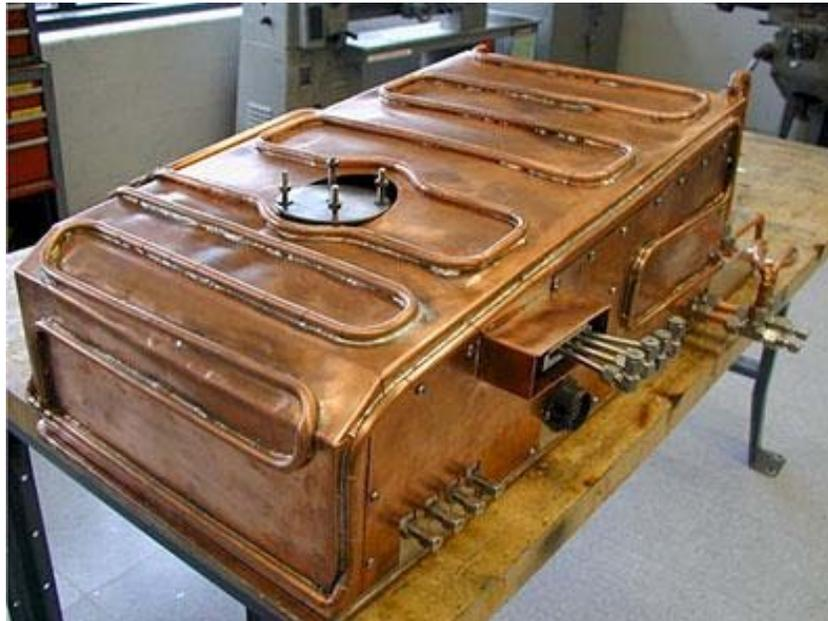
**Figure 3-4. Photograph of the inverted-pendulum thrust stand with water-cooled shroud.**
