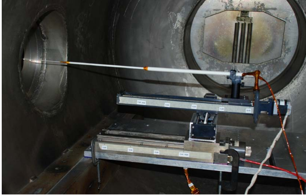
Figure 4.19. Langmuir probe setup for internal measurements.
