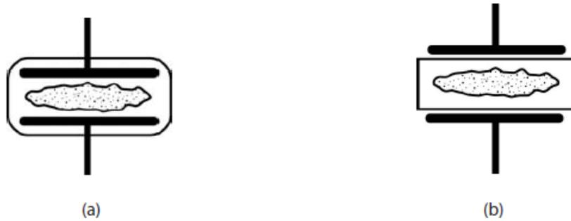
Figure 3.3: Configurations for capacitive discharges: a) electrodes inside the plasma, and b) electrodes outside the plasma [37].
