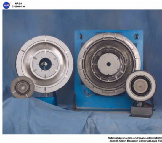
Figure 2.7: Hall-effect thrusters developed by NASA ranging from 3 kW to 50 kW nominal power. Photo courtesy of NASA.
