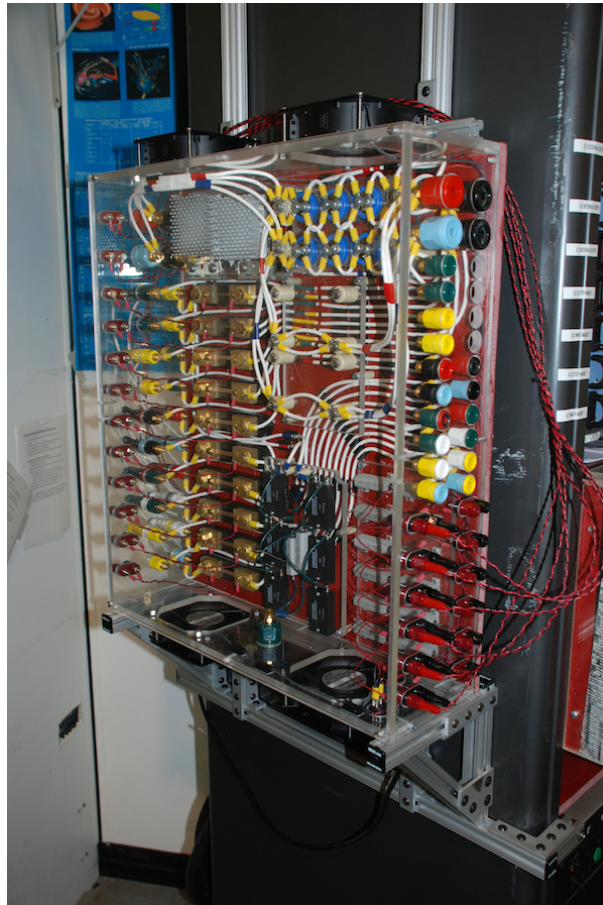
Figure 3.10: Enclosure housing the discharge filter, current shunts, voltage dividers, and protection diodes
