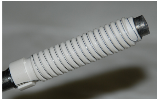
Figure 3.3: Updated heater on the second \text{LaB}_6 cathode.
