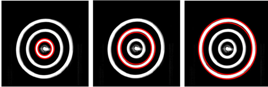
Fig. 2 Example ellipses fit to identify the inner (left), middle (center), and outer (right) discharge channels from the same mean image. This technique was applied to all multichannel conditions to isolate each channel.
