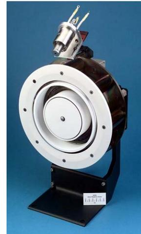
**Figure 2. NASA-173Mv1 Hall Thruster**
