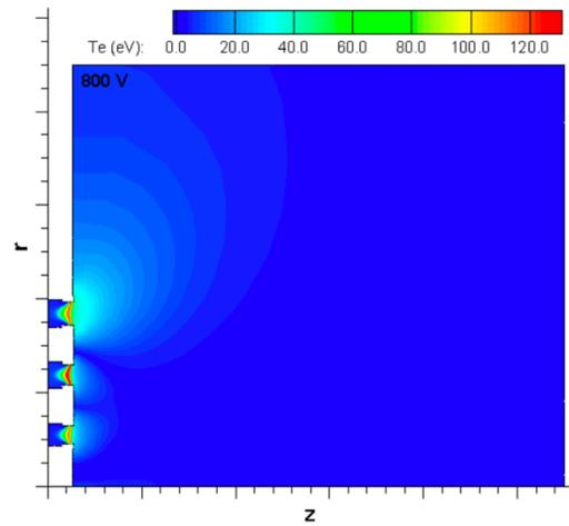
Figure 4: Sample of output from simulation of the X3 generated by JPL's thruster code, Hall2De. The data shown is electron temperature at the 800 V, 100 kW condition. Figure taken from Ref. [11].
