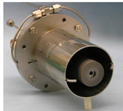
*Figure 1: 250-A class  $\text{LaB}_6$  hollow cathode from NASA JPL with external flow injectors*
