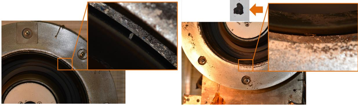
**Figure 47. (left) Close-up and location of “1:30” carbon flake found between discharge channel and outer screen (post-Phase C). (right) Close-up and location of “6:00” (“Ohio” shaped) carbon flake found between discharge channel and outer screen (post-Phase C).**
