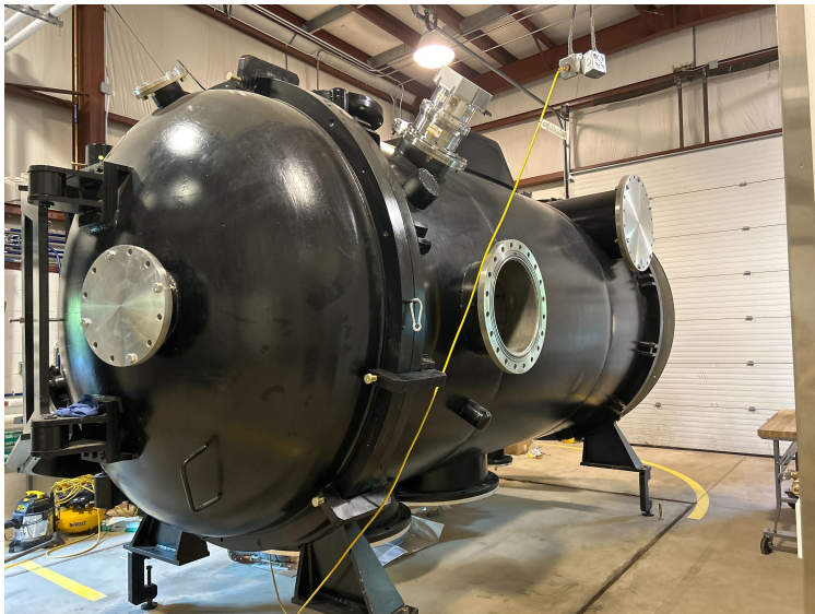
Figure 9: Alternative propellant test facility (APTF) at the University of Michigan.
