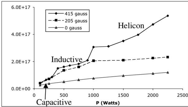
**Figure 3.** Ion number density as a function of input power and peak magnetic field strength, probe location: (0,0), chamber pressure: 5 mTorr
