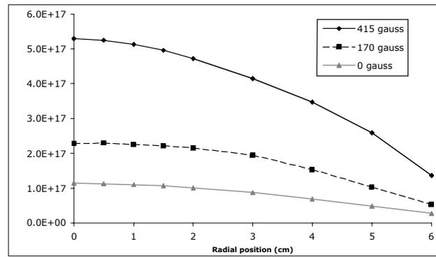
**Figure 5.** Ion number density as a function of radial position and magnetic field strength, axial position: 0 cm, input power: 1750 watts, chamber pressure: 1 mTorr
