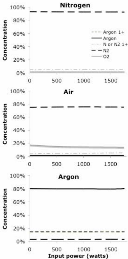
Figure 6. Molar concentration as a function of input power as measured by the RGA for various species.
