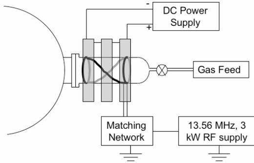
**Figure 2.** Electrical setup of PEPL helicon source with DC magnets and RF antenna.
