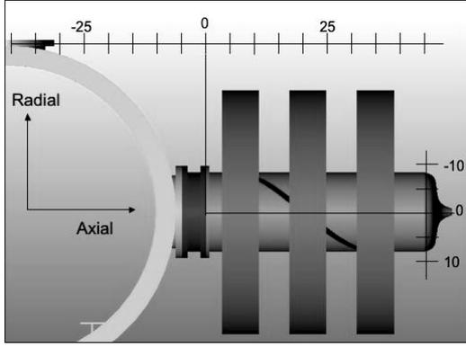
**Figure 1.** PEPL helicon source layout with dimensions. Units are in cm. The (0,0) location is located where the quartz tube meets with the CTF flange, in the radial center of the quartz tube. Magnets and antenna can be seen surrounding the quartz tube.
