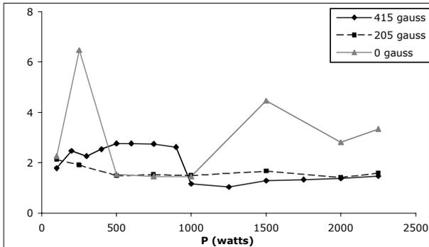
**Figure 4.** Electron temperature as a function of input power and peak magnetic field strength, probe location: (0,0), chamber pressure; 5 mTorr
