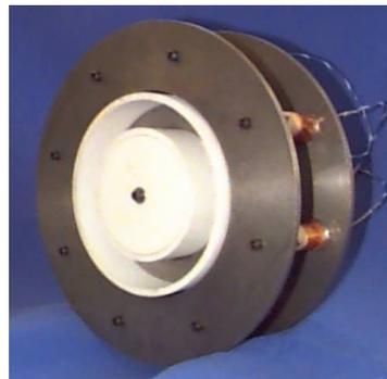
Figure 2, P5, 5 kW class laboratory model Hall thruster.
