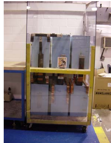
Figure 7. Photograph of the 16 kJ G capacitor bank. Not included in this photograph is the later-added RF shielding, and full kinetic shielding infrastructure.
