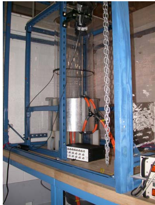
Figure 4. Photograph of the coils mounted in the E/M shielding cage, power supplies, and general facility setup. Note the vertical configuration of the coil/chamber assembly.
