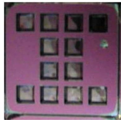
Figure 10: First-generation MEMS gate design showing the viewing windows etched into the bulk silicon. Each viewing window contains tens of thousands of emission channels. The current MEMS gate is a second-generation design.
