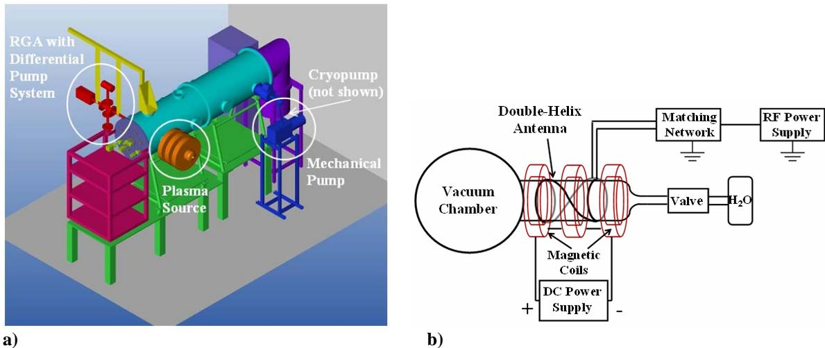
Figure 1. a) Main vacuum chamber setup. b) Schematic diagram of plasma source.
