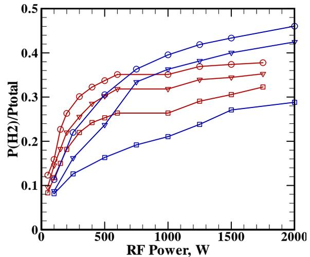
**Figure 7. Ratio of H<sub>2</sub> partial pressure to total pressure at a) 1 mtorr (blue lines), 200 mtorr (purple lines), 300 mtorr (green lines), and 400 mtorr (red lines) and b) 400 mtorr (red lines) and 1 mtorr (blue lines) chamber pressure. Applied DC current to the magnetic coils are 0 A (square), 30 A (triangle) and 60 A (circle).**
