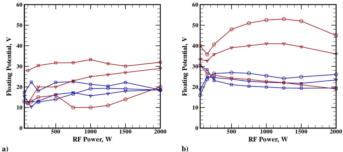
**Figure 4. Floating potential current versus RF power for a) 1 mtorr chamber pressure and b) 100 mtorr chamber pressure. Applied DC current to the magnetic coils are 0 A (square), 30 A (triangle) and 60 A (circle) for argon (blue lines) and water vapor (red lines).**
