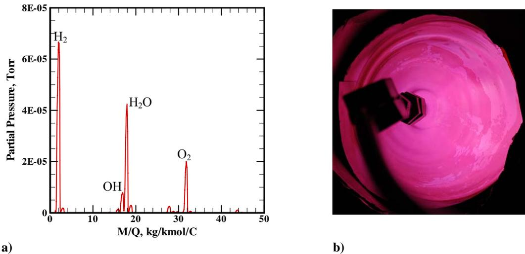
Figure 5. a) A sweep of raw RGA data. b) Picture of water plasma at 1 mtorr, 60 A, and 1.5 kW.
