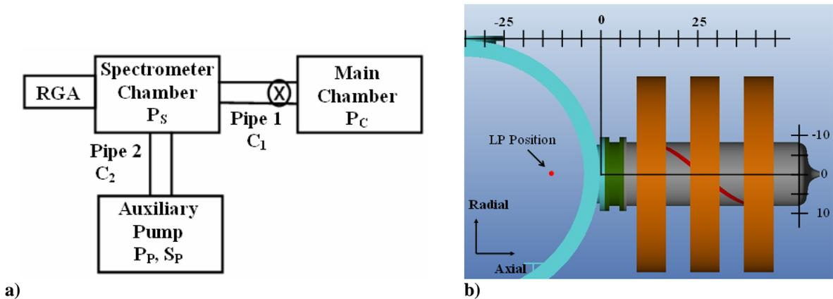
**Figure 2. a) Schematic diagram of differentially pumped system for the RGA. b) Plasma source with axis definition. Langmuir probe data are taken at -13 cm in the axial direction.**
