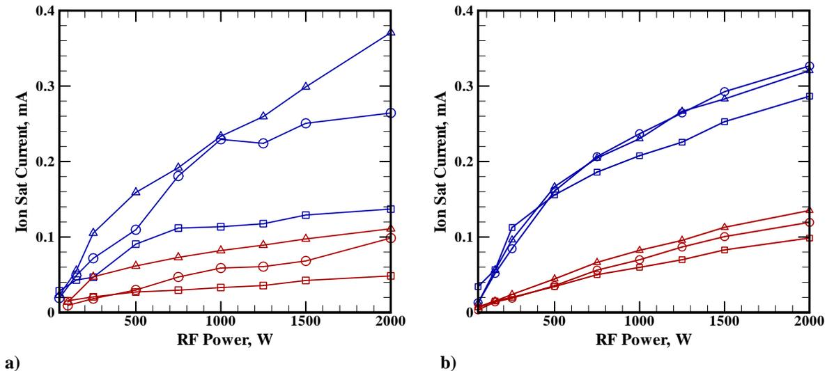
Figure 3. Ion saturation current versus RF power for a) 1 mtorr chamber pressure and b) 100 mtorr chamber pressure. Applied DC current to the magnetic coils are 0 A (square), 30 A (triangle) and 60 A (circle) for argon (blue lines) and water vapor (red lines).
