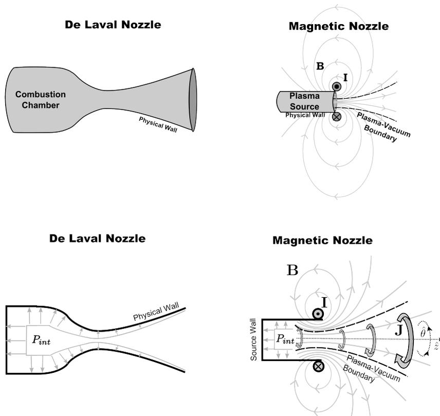
Figure 2. De Laval nozzle compared to magnetic nozzle produced by current loop with current  $I$ .
