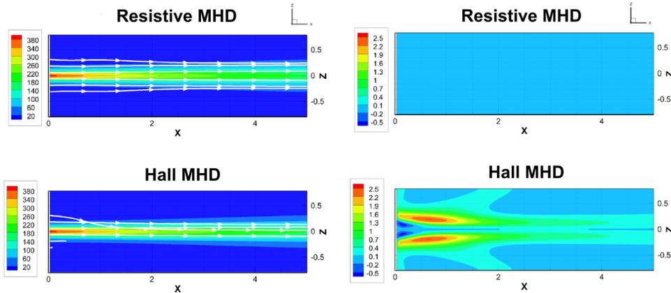
Figure 8. Left: Contours of axial velocity and velocity streamlines, Right: Contours of azimuthal ( $\hat{\theta}$ ) velocity (m/s)
