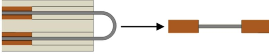
Figure 27. The hairpin filament geometry is simplified to a purely linear geometry with a planar material interface in the 1D finite element model.
