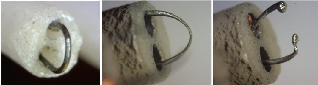
Figure 2. Evaporative mass loss leads to emissive probe failure. Left, a virgin filament mounted in a dual-bore alumina tube. Middle, a filament intact after testing but showing preferential mass loss at the hottest region, the tip. Right, a filament destroyed during testing. In the moment of failure the temperature runs away leading to globules of melted tungsten at each end.
