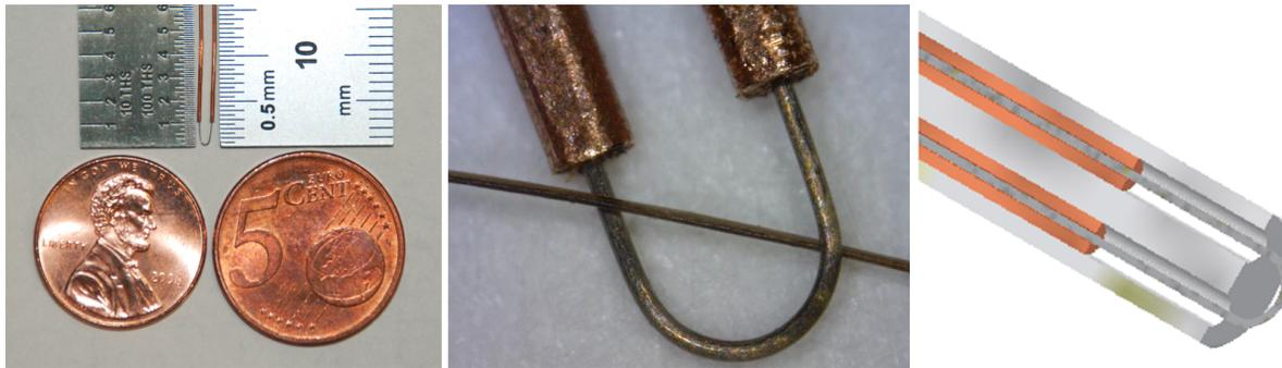
**Figure 4. Example of a 0.1 mm diameter (.004”) emissive probe filament with crimped copper tubes for lead wires. From left, a filament used for plume mapping with 2.5 mm exposed filament from tip to copper junction; middle, a filament shown in extreme closeup with a human hair overlaid for scale (this filament not used for testing); right, a CAD cutaway showing the filament with copper tube leads in a 1.6 mm OD dual-bore alumina tube.**
