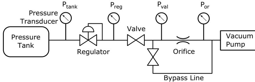
**Figure 6: A schematic of the propellant feed system characterization experimental setup.**
