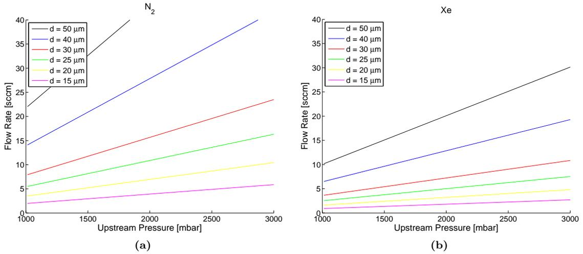
**Figure 4: The nominal expected mass flow rate of a) nitrogen and b) xenon through a given COTS orifice size with the range of pressures upstream of the orifice that the pressure regulator can deliver.**
