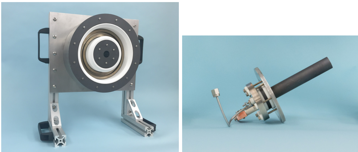
Figure 2 Left – The H9 magnetically shielded Hall thruster, shown without a cathode. Right – The LaB 6 hollow cathode that is mounted on thruster centerline in the H9.
