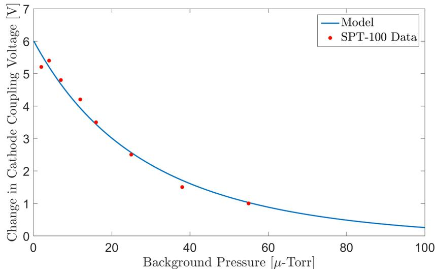
Figure 4: Plot showing the results of simulating equation 13 versus SPT-100 data inferred from Diamant.<sup>34</sup> The results shown are changes in the coupling voltage not the absolute voltage.
