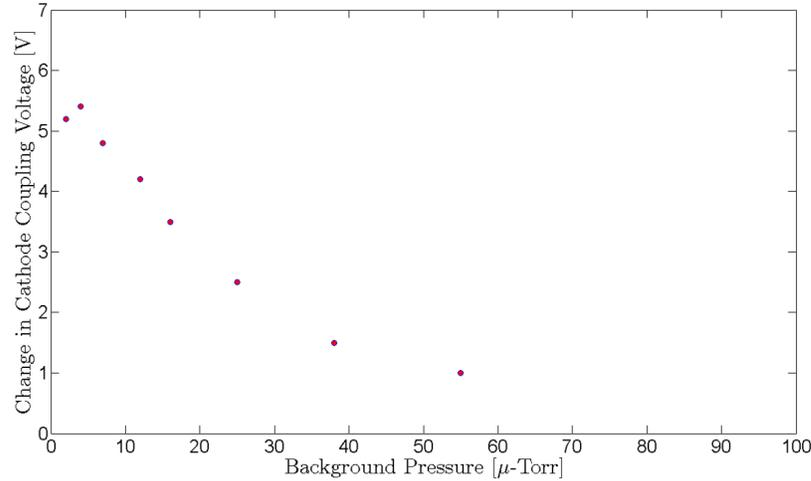
Figure 3: Change in cathode coupling voltage as a function of background pressure. This data was inferred from cathode to ground and plasma potential measurements, not directly measured<sup>29</sup>
