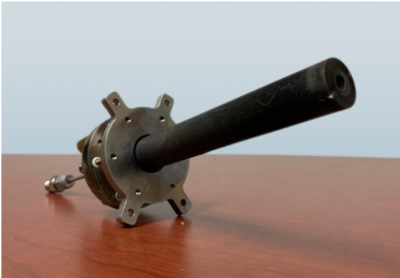
Figure 2: H9 LaB 6 hollow cathode
