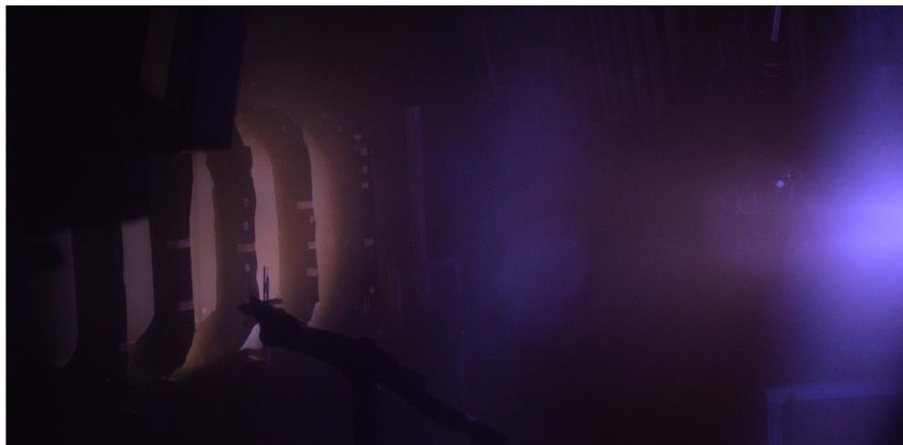
**Figure 18. Photograph of the beam catcher operating at 5 A solenoid current 100 V bias (left) in the presence of an H9 thruster beam (right).**
